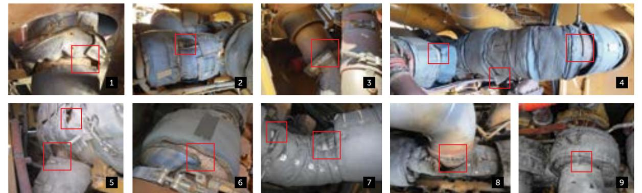
**PHOTOS 1-9** Assess poor fitment alongside blanket condition. Fix gaps (5,7) and assess if fit-for-purpose. Replace overworn and baggy-fit blankets (2,4,8). Replace damaged blankets and missing sections (3,6,9). Consider upgrading tie-wire to springs for a snug fit (1,2).
