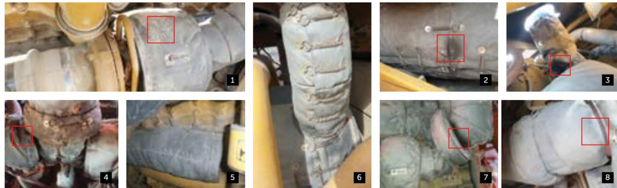
**ABOVE** Residual dirt build-up and low-level soot are typical (1,2,6). Investigate prominent soot on blankets for engine pipe leaks (3,7). Eliminate gaps and refit blankets (8) for a snug-fit and maximise coverage (4). Monitor blanket condition during ongoing maintenance.
