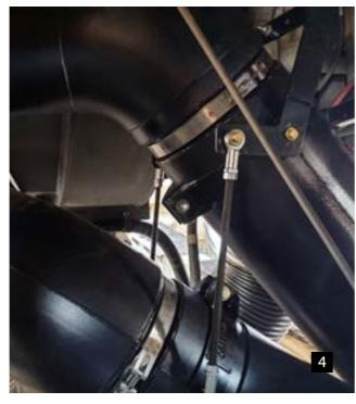
**ABOVE** Liebherr T282C dual-wall exhaust system, engine pipe and mounting details. Thermal blankets installed on turbos.
