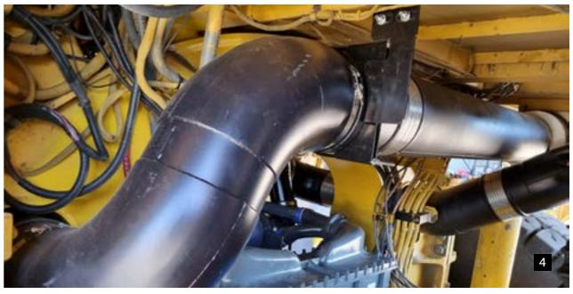
ABOVE Komatsu 830E-AC dual-wall exhaust system, engine pipe and mounting details.
