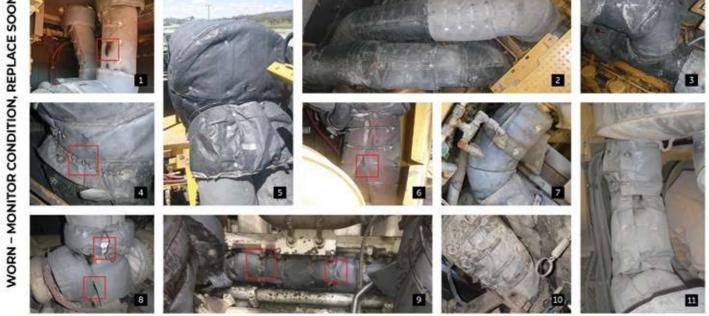
ABOVE Fix and refit blankets to avoid hot spots from gaps (1,6,8). Refit/replace stretched springs and loose tie-wire (4,6,8). Monitor and schedule replacement for wear (9), soot marks (2,3,8-11) and irreparable/loose fitments (8). Investigate burn marks for exhaust leaks (1,8).
