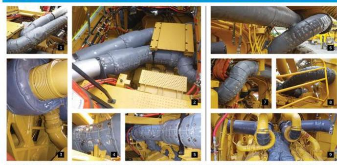
PHOTOS 1-5 Cat 793F manifold, turbo, junction, e/pipe blankets PHOTOS 6-9 Komatsu 830E manifold, turbo, junction, e/pipe blankets
