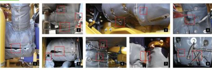
PHOTOS 1-8 Poor fitment (1,3,8), excessive gaps (2-5,7), and poor install techniques (8) create hot spots. Eliminate gaps and ensure blankets are snug-fitting and maximise coverage. Check springs are connected, tie-wires secured, and replace missing springs.
