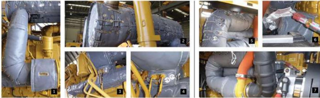
PHOTOS 1-4 Cat D11T manifold, turbo, e/pipe and muffler blankets PHOTOS 5-7 Cat 815K manifold, turbo and e/pipe blankets
