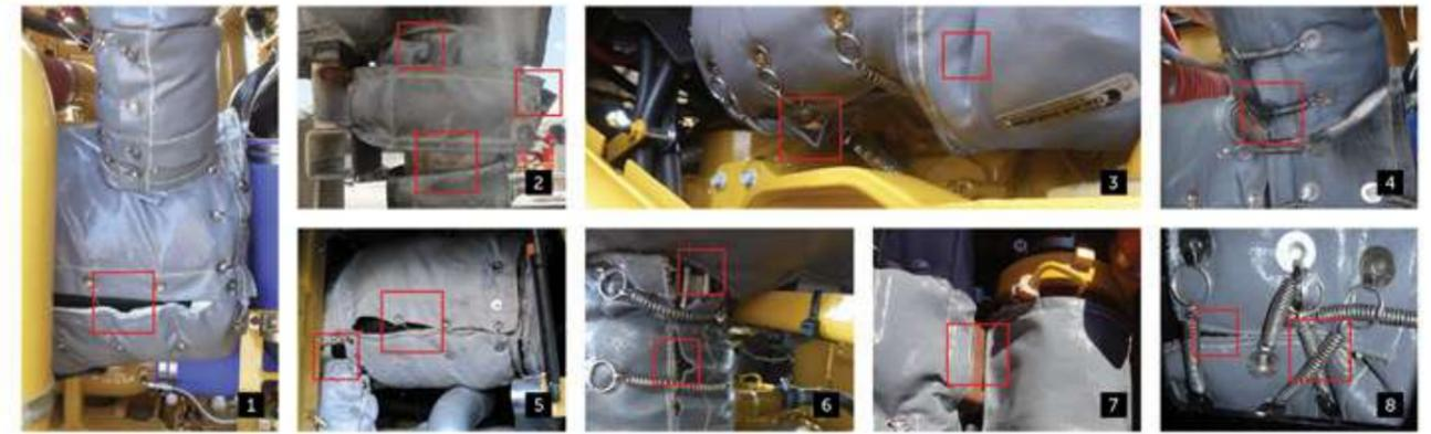
**PHOTOS 1-8** Poor fitment (1,3,8), excessive gaps (2-5,7), and poor install techniques (8) create hot spots. Eliminate gaps and ensure blankets are snug-fitting and maximise coverage. Check springs are connected, tie-wires secured, and replace missing springs.
