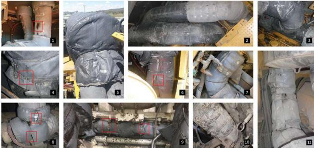
**ABOVE** Fix and refit blankets to avoid hot spots from gaps (1,6,8). Refit/replace stretched springs and loose tie-wire (4,6,8). Monitor and schedule replacement for wear (9), soot marks (2,3,8-11) and irreparable/loose fitments (8). Investigate burn marks for exhaust leaks (1,8).
