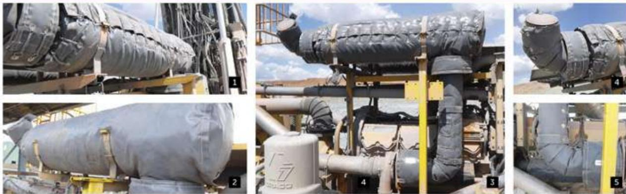
PHOTOS 1-5 Atlas Copco PV275 turbo, engine pipe, muffler and tailpipe blankets. Manifold blankets available (not pictured).
