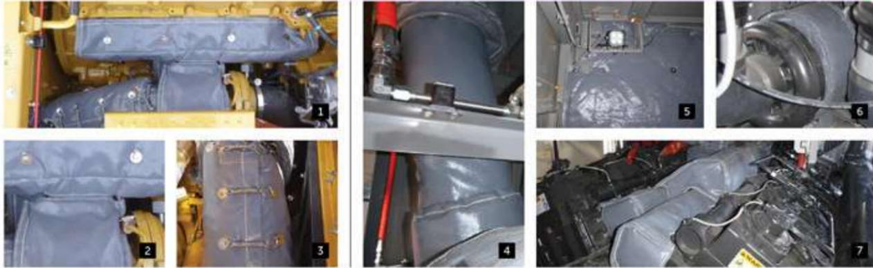
PHOTOS 1-3 Cat 336 manifold, turbo and e/pipe blankets PHOTOS 4-7 Hitachi 5600-6 manifold, turbo, e/pipe and firewall blankets
