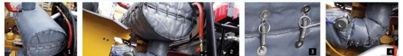
PHOTOS 1-4 Cat 966M turbo, engine pipe, muffler and tailpipe blankets. Manifold blankets available (not pictured).
