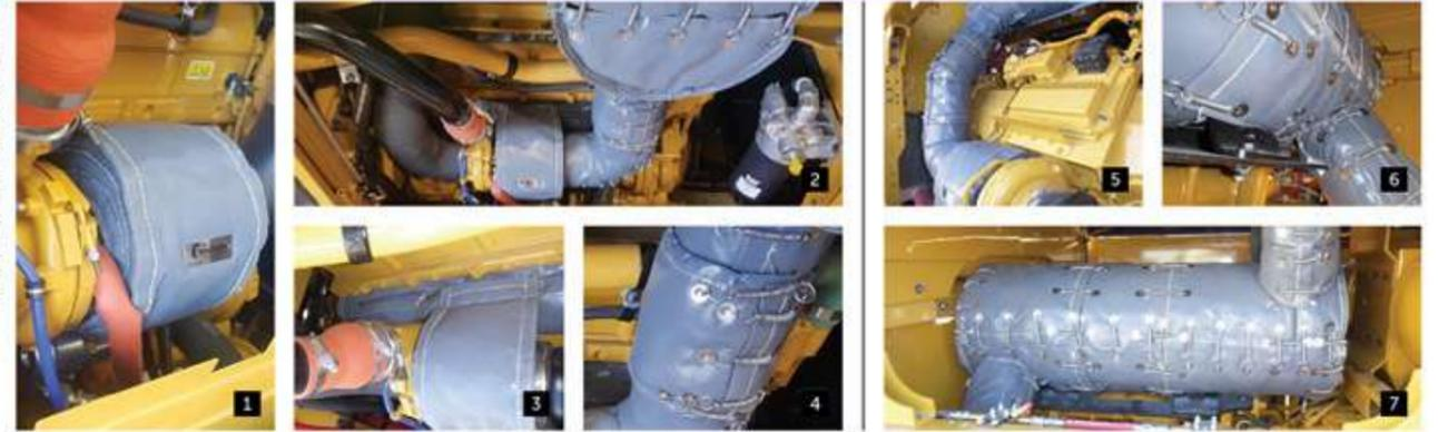
PHOTOS 1-4 PHOTOS 5-7 Cat 24 manifold, turbo, e/pipe, muffler, t/pipe blankets
