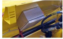
Data logger records backpressure, exhaust gas temperature and engine RPM
