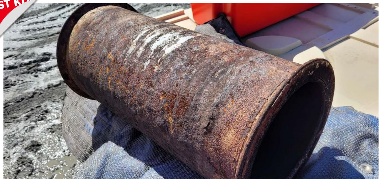
Aletek exhaust components after 6 years. Surface rust, but intact and remain fit for purpose.
