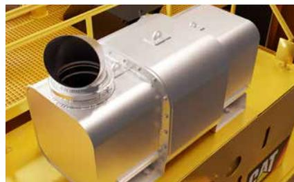
DPF replaces the factory-fitted DPF using existing mounting points
