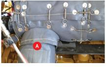
**MUFFLERS** Open blanket and wrap around muffler. Connect springs to anchors. Ensure inlet flange is installed over engine pipe cover (A). Massage blanket to final shape for best coverage.
