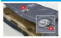
MANIFOLDS Attach tie wire end to anchor (A). Hold blanket against manifold. Feed wire behind manifold cylinder runners. Massage blanket to final shape. Loop wire around anchor, connect springs to anchors (B).
