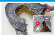
**TURBOS** Feed wire through spring keyring to work as a pull-wire (A). Open turbo shell (B). Slide blanket over turbo. Pat blanket to fit shape. Ensure oil line is outside the blanket to prevent overheating and oil line damage (C).
