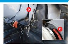
Connect springs on blanket. Remove pullwire from keyring. Ensure blanket mates to manifold blanket, maximise coverage. Pat blanket into position. If the outlet flange cover is fitted ensure this section is outside engine pipe blankets (D).
