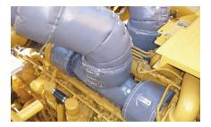
**JUNCTIONS** Open blanket and wrap around junction. Connect centre spring and work outwards connecting springs. Massage blanket to final shape for best coverage.
