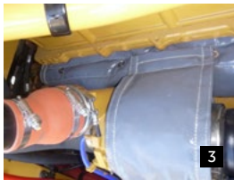
PHOTOS 1-7 Cat 24 manifold, turbo, e/pipe, muffer, t/pipe blankets
