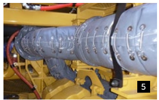
PHOTOS 1-5 Cat 793F manifold, turbo, junction, e/pipe blankets PHOTOS 6-9 Komatsu 830E manifold, turbo, junction, e/pipe blankets
