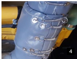
PHOTOS 1-7 Cat 24 manifold, turbo, e/pipe, muffer, t/pipe blankets
