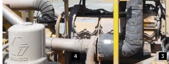
PHOTOS 1-5 Atlas Copco PV275 turbo, engine pipe, muffler and tailpipe blankets. Manifold blankets available (not pictured).
