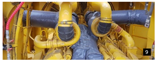
PHOTOS 1-5 Cat 793F manifold, turbo, junction, e/pipe blankets PHOTOS 6-9 Komatsu 830E manifold, turbo, junction, e/pipe blankets
