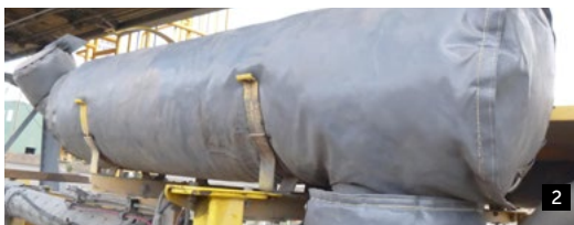
PHOTOS 1-5 Atlas Copco PV275 turbo, engine pipe, muffler and tailpipe blankets. Manifold blankets available (not pictured).
