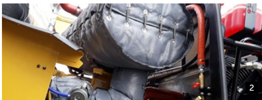
PHOTOS 1-4 Cat 966M turbo, engine pipe, muffer and tailpipe blankets. Manifold blankets available (not pictured).
