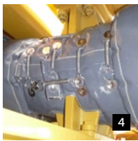
PHOTOS 1-5 Cat 793F manifold, turbo, junction, e/pipe blankets PHOTOS 6-9 Komatsu 830E manifold, turbo, junction, e/pipe blankets
