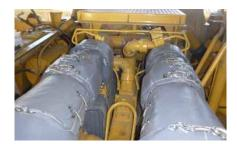
Thermal blankets are integral for effective fire mitigation in engine bays
