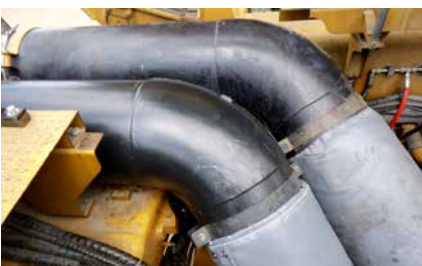
Thermal blankets are integral for effective fire mitigation in engine bays
