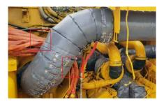
Add blankets to protect high voltage lines against contact with hot exhaust surfaces
