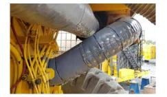
Thermal blankets are integral for effective fire mitigation in engine bays
