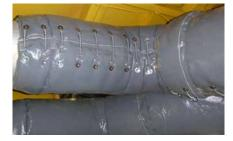
Add blankets to engine pipes to mitigate engine fire risks
