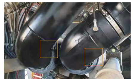
Add blankets to turbos, manifolds and junctions to mitigate engine fire risks
