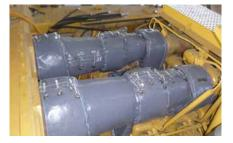
Mitigate the risk of engine fires by adding blankets to heat critical components
