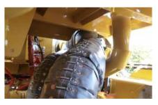
Mitigate the risk of engine fires by adding blankets to heat critical components
