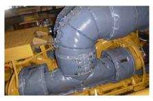
Mitigate the risk of engine fires by adding blankets to critical heat components
