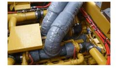
Mitigate the risk of engine fires by adding blankets to heat critical components
