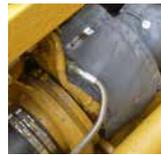
Add blankets to turbos, manifolds and junctions for fire mitigation
