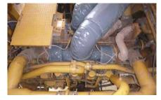
Mitigate the risk of engine fires by adding blankets to critical heat components
