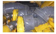
Mitigate the risk of engine fires by adding blankets to critical heat components
