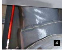
PHOTOS 1-3 Cat 336 manifold, turbo and e/pipe blankets PHOTOS 4-7 Hitachi 5600-6 manifold, turbo, e/pipe and firewall blankets
