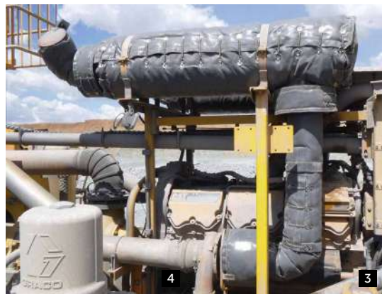
PHOTOS 1-5 Atlas Copco PV275 turbo, engine pipe, muffer and tailpipe blankets. Manifold blankets available (not pictured).
