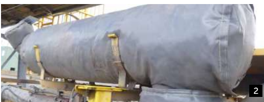
PHOTOS 1-5 Atlas Copco PV275 turbo, engine pipe, muffer and tailpipe blankets. Manifold blankets available (not pictured).
