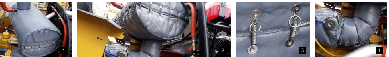
PHOTOS 1-4 Cat 966M turbo, engine pipe, muffler and tailpipe blankets. Manifold blankets available (not pictured).
