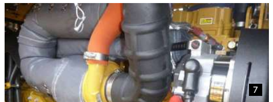
PHOTOS 1-4 Cat D11T manifold, turbo, e/pipe and muffler blankets PHOTOS 5-7 Cat 815K manifold, turbo and e/pipe blankets
