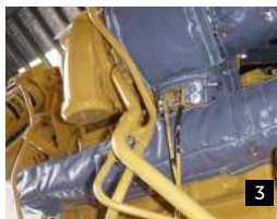
PHOTOS 1-4 Cat D11T manifold, turbo, e/pipe and muffler blankets PHOTOS 5-7 Cat 815K manifold, turbo and e/pipe blankets
